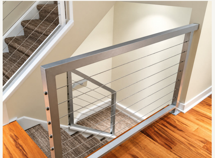
2 x 2 Aluminum Square Frame with 1/8 in. stainless steel cables. Anodized Silver.
